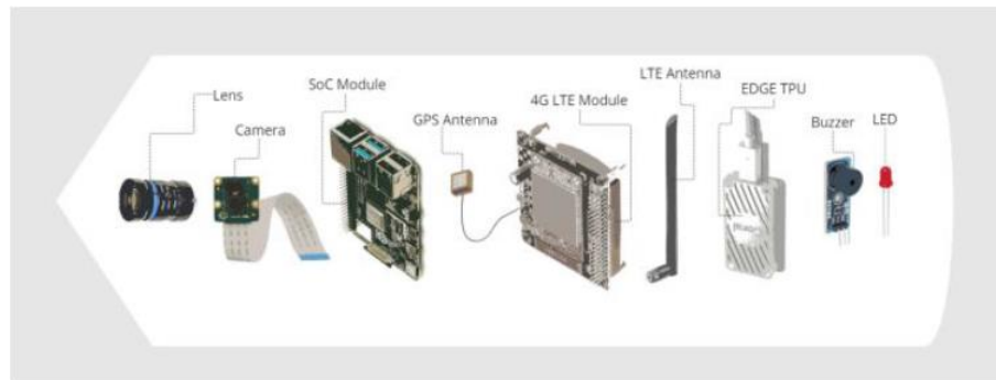
Figure 3: Device hardware components.
